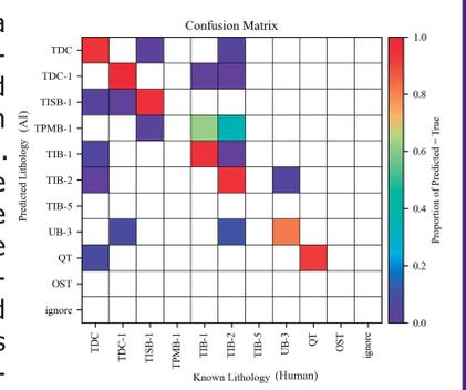
**Fig. 10:** DHK-27 confusion matrix visualizing the performance of supervised learning algorithm versus the geologist selected intervals used in the AI training. Source: GeologicAI.
