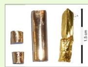
Starting materials were natural basaltic andesite and dacite from the most recent eruptions of Volcán Quizapu in Chile, the compositions of which have been fully characterized and reported (Fiege et al., 2017; Ruprecht et al. 2012). Prior to each diffusion-couple experiment, the mafic and felsic starting materials were equilibrated separately and then juxtaposed in a single capsule, with the less dense felsic material overlying the mafic material.
