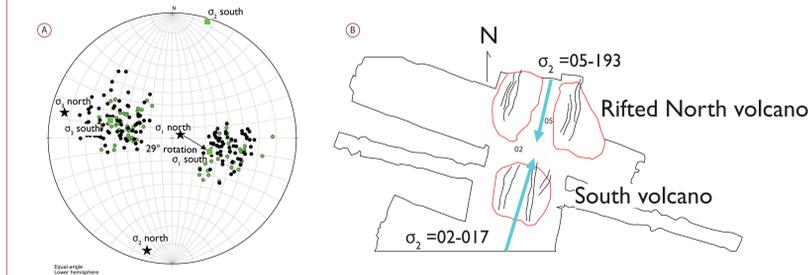
Figure 5. A) Stereonet of poles to fault planes in the northern rift (black circles) and in the southern rift (green circles). Arrow shows a clockwise rotation of 29° from the northern rift to the southern rift. Stress orientations in black stars (northern rift) and green squares (southern rift). B) Sketch of study area highlighting slight variations in  $\sigma_1$  trend as well as plunge, both plunge towards the bathymetric low between the volcanic edifices.
