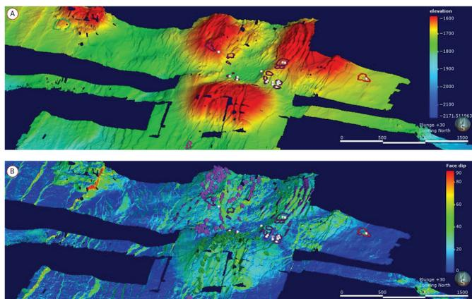
Figure 3. A) Oblique view (30°) of bathymetric map from the central area of Lucky Strike, resolution is ~1m, hydrothermal sites are in polygons, white points are sampled sites. B) Dip face map used to determine structural measurements and individual measurements are in circular features, purple for the northern part of the rift and green in the southern part of the rift.
