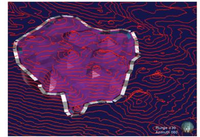
Figure 8. A) Example of volume estimation for the massive sulfide deposits at the site Sintra. Contours every 2 meters (red) and outline of the deposit (gray). B) Location of the site in A).
