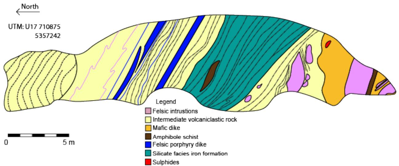
**Figure 3.** Road-cut outcrop map along strike of the Cubric showing; vertical section faces west.
