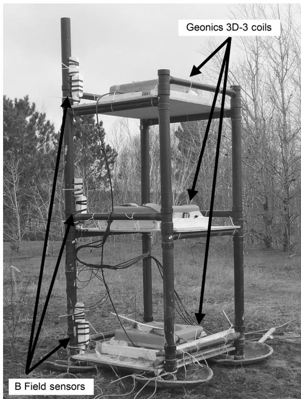
Figure 6. Vertical spatial derivative measurement structure made of PVC pipe and wood housing three Geonics 3D-3 coils ( $x$ ,  $y$ , and  $z$  components) and three vertical B-field feedback sensors with each level separated by 1.1 m. The apparatus was dragged from station to station.
