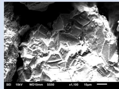
Figure 4.1: SEM Uncleaned Sample Grains (after HCl pre-leach, before nitric)
