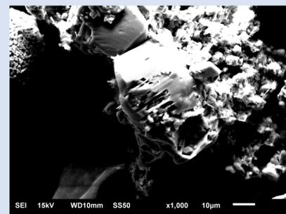
Figure 4.2: SEM Cleaned Sample Grains (after HCl pre-leach and nitric)
