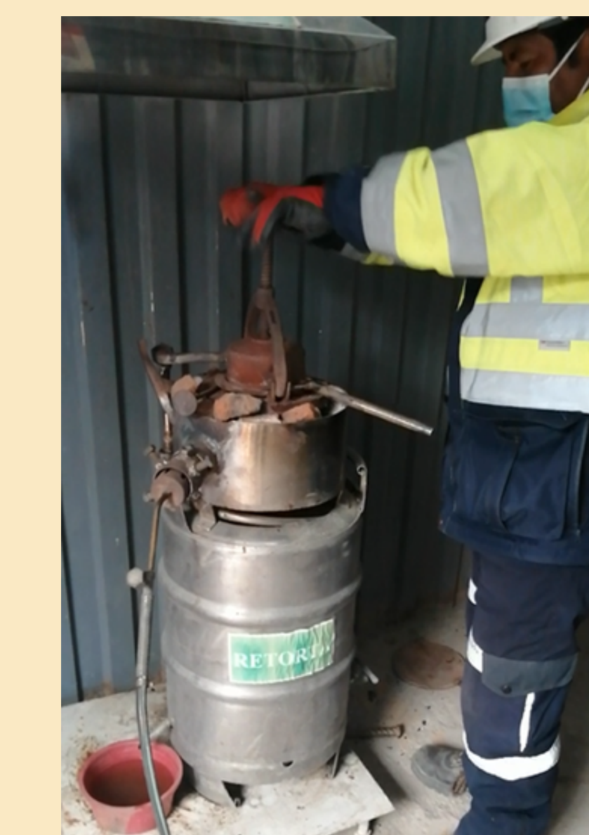
Retort and furnace for vaporizing mercury at Cruz Pata Chiquimas
