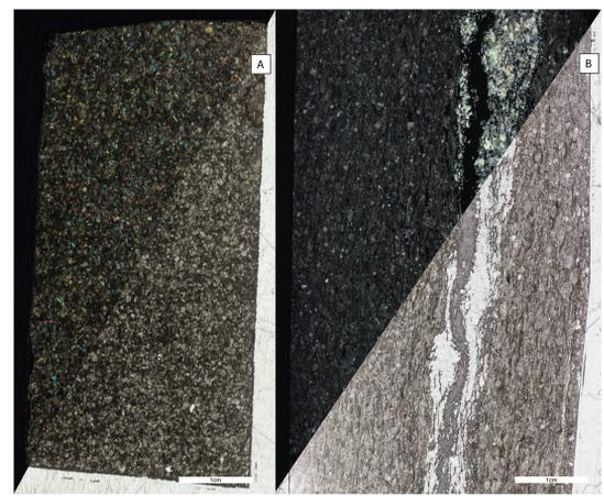
The enriched Mg-Cr-Ni unit largely consists of amphibole, chlorite, biotite, and plagioclase with minor ilmenite, epidote, talc, apatite, and quartz. Accessory phases include titanite, chromite, and zircon. The Timiskaming metagreywacke consists of quartz, plagioclase, and biotite with accessory amphibole.
