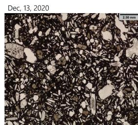
These petrographic images were produced through imaging under PPL, accompanied by stitching using FIJI. A total of 25 images were taken and stitched together for each sample, in hopes of facilitating morphological analysis. Bubble and crystal size distribution (CSD) were to be done once high quality images were produced.
