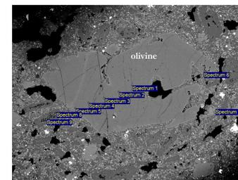
Sample 010421F: Spectrum 7 corresponds to a pyroxene grain, while Spectrum 6,8-9 correspond to plagioclase grains.
