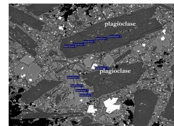
Sample 160221F: Spectrum 6-9 corresponds to pyroxene groundmass, while spectrum 10 corresponds to titanomagnetite oxide.
