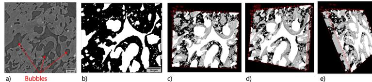
Sample 210821A: Preparation and final visualization of tomography images. a) shows a selected axial slice in its initial form; b) shows the same slice in 8-bit and with the segmentation of the bubbles. c), d), and e) show 3D visualizations of these bubbles. In a), the bubbles are labeled, while in b), the bubbles are white. In 3D visualizations (c-e), a sub-volume of the imaged sample is shown, where the white content are the bubbles within the ash sample.
