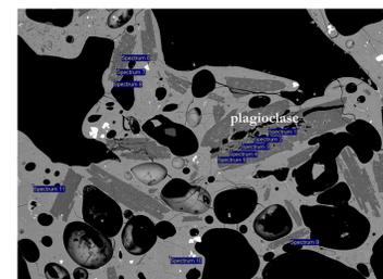
Sample 160221L: Spectrum 1-9 corresponds to plagioclase phenocrysts, while Spectrum 10,11 capture the matrix.
