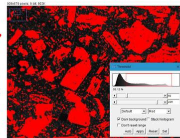
Upon completion of image production, it was found that CSD was a challenge in the flow samples, as FIJI was not able to properly segment the differing crystal species. As seen to the right, thresholding of the image to begin CSD would require days of manual manipulation to produce a viable sample for analysis.
