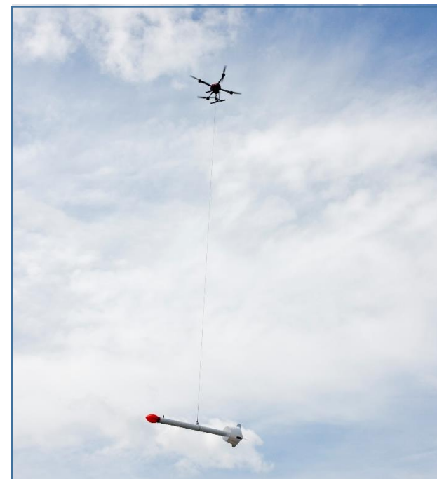
UAV-Ground Mag/EM system
