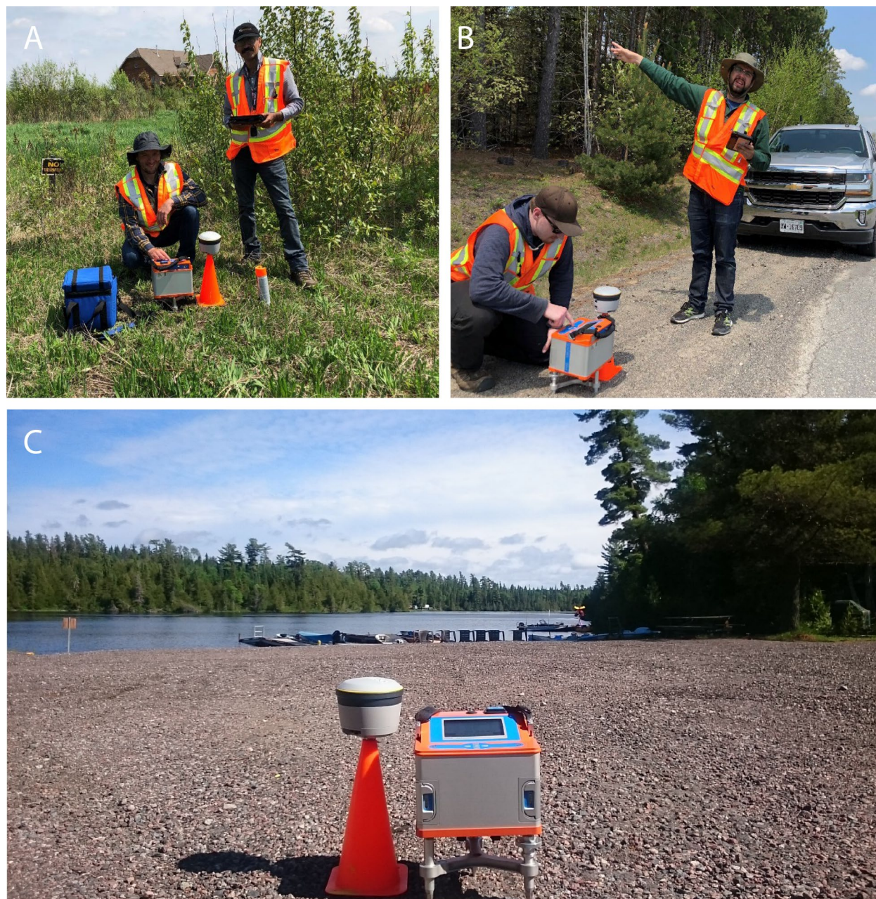
Photo 46.1. A, B) Geophysical field crews collecting gravity data and petrophysical samples in summer 2018. C) Scintrex CG-6 Autograv™ gravity meter (right) and a Trimble® R2 GNSS receiver (left) used in the collection of the gravity data.
