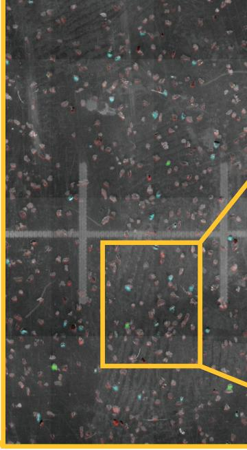
$\mu$ XRF elemental map of HMCs with Fe, Ti, and P elemental abundance overlayed Bright green, blue, and red indicates apatite, rutile, and magnetite respectively.
