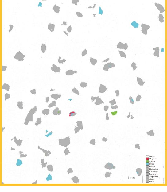
Inset µXRF elemental map with P, and Ti el- ASEM-EDS mineral map of the µXRF inset area Apatite and rutile readily identifiable by  $\mu$ XRF elemental maps and SEM-EDS automated mineralogy
