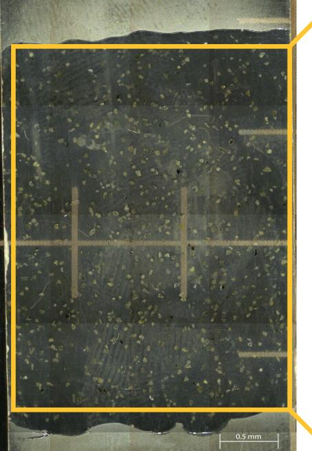
Mosaic RGB image of till derived heavy mineral concentrates (HMC) mounted in epoxy in a polished thin section.
