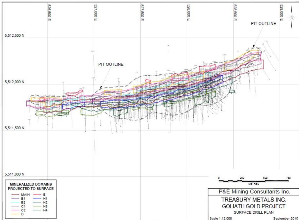
**Fig. 6** – Plan view of the major mineralized domains delineated within the Goliath Deposit with the outline of the proposed open pit indicated (from Puritch et al., 2015).
