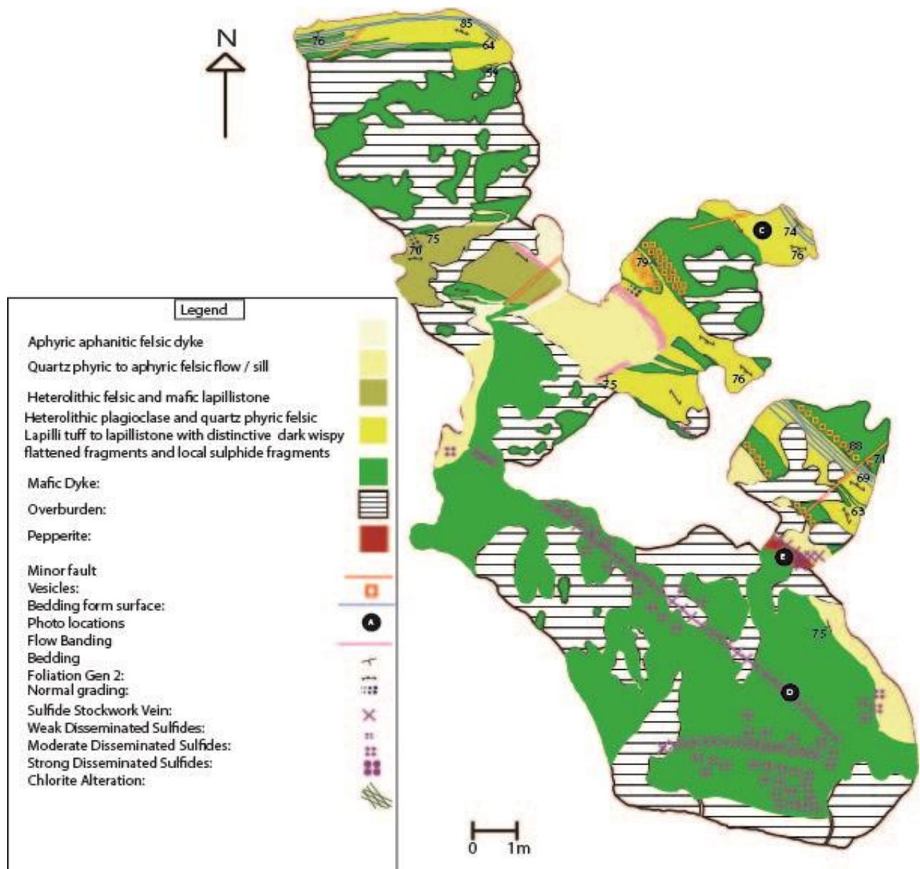
**Figure 5:** Stop 3 – outcrop map showing lithology, structure and alteration and photo locations C, D, E. Interpretation
