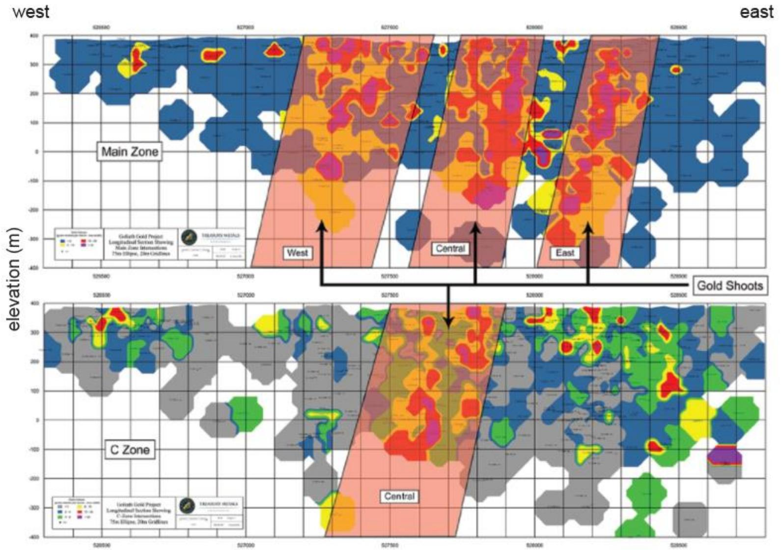
**Fig. 5** – Longitudinal section through the Main and C Zones of the Goliath Deposit showing the westerly plunge of the high-grade ore shoots (from Puritch et al., 2015).
