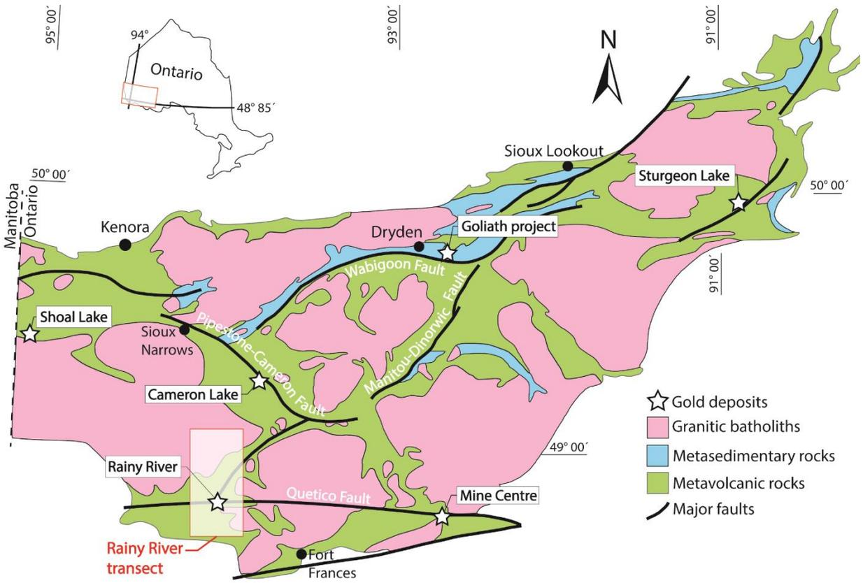
**Figure 1** Simplified geological map of the western Wabigoon subprovince displaying the location of the main Au deposits and prospects (modified from Blackburn et al., 1991).
