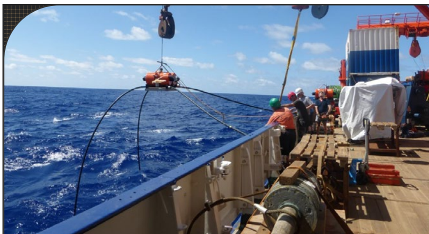
Figure 3: Image of one of 18 ocean bottom magnetotellurics (OBMT) stations that were deployed and left on the seafloor, during a period of 41 days, to collect research data.
