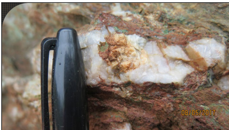
Figure 14: Gold mineralization in a quartz vein hosted in fuchsite carbonate altered ultramafic rocks from the Kerr Addison Mine.
