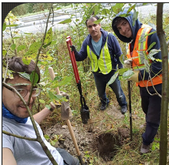
Figure 27: Metal Earth seismic group planting passive seismic receivers in Larder Lake, Ontario. L-R: Christopher Mancuso, Dr. Saeid Cheraghi, and Hossein Jodeiri Akbari Fam.
