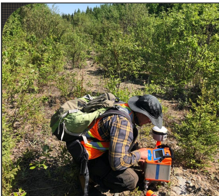
Figure 28: Fabiano Della Justina acquiring gravity data using a Scintrex CG-6 gravity meter and Trimble R2 GPS receiver.
