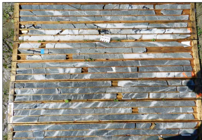
Figure 1. High-grade intersection of the 58N zone, with brittle stockwork-type quartz ± carbonate ± tourmaline veins in a porphyry intrusion with silica, sericite, and biotite alteration.
