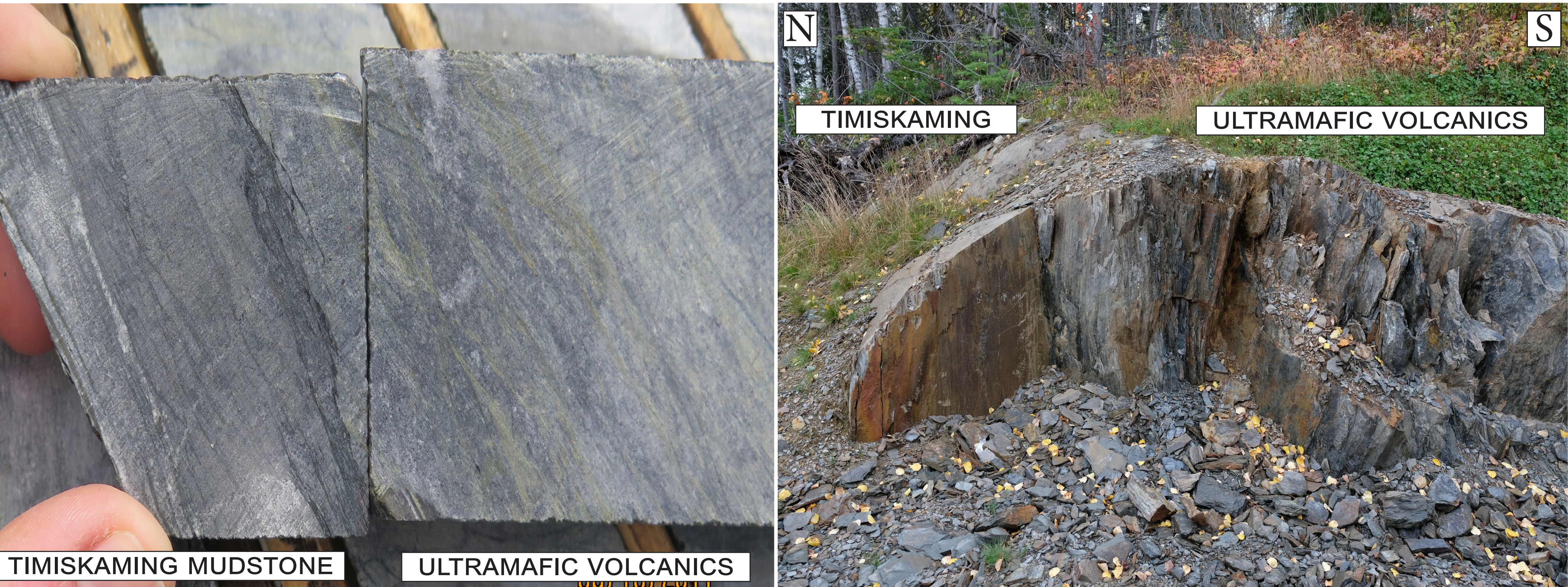
Figure 4. Contact between Timiskaming sediments and Larder Lake Group ultramafic volcanics in drill core (left, NQ drill core) and outcrop (right, west of Virginiatown, Ontario). Location: 604824E 5332042N (UTM co-ordinates are in NAD83, Zone 17N).
