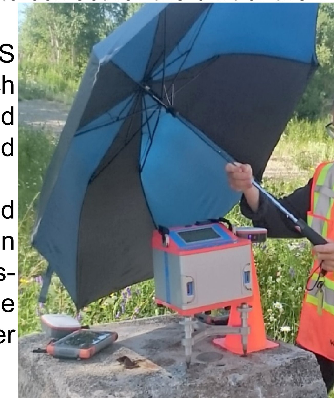
Fig.3. The CG-6 Gravimeter and Juniper system Geode collecting data on Chibougamau base station
